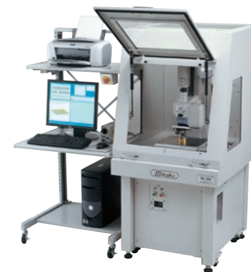
Model: NH-3SP (Super precision model) Measuring range: XYZ = 150mm X 150mm X 10mm Scale resolution: XYZ = 0.01μm, 0.01μm, 0.001μm Applications: aspherical lenses, semiconductors, precision molds, etc.
