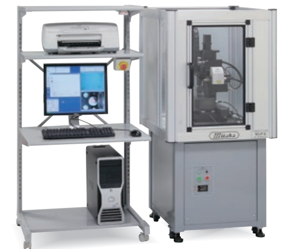
Model: MLP-2 (360-degree measurement model) Measuring range: XYZ = 120mm X 90mm X 130mm AF (R) = 40mm, AZ (θ) = 360° Scale resolution: XYZ = 0.1μm, 0.1μm, 0.1μm AF (R) = 0.01μm, AZ (θ) = 0.001° Applications: precision gears, endmills, punches, molds for connectors, etc.
